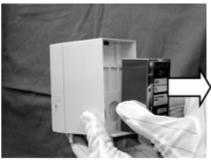
5. Insert the new sensor unit, then reattach the main body cover.
