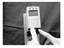
Pull the two latches at the bottom of the base unit back, and (while they are still pulled back) release the main unit, pulling from the top.
