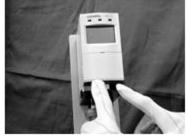
2. Pull the cover lock knob down and release the lock. After pulling it down further below, pull back the pyrolyzer case cover and remove it.
